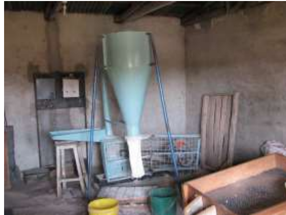
Photo 8 Feed manufacture equipment; sifter, mixer, pelleter
