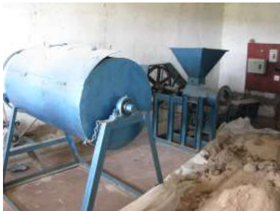
Photo 8 Feed manufacture equipment; sifter, mixer, pelleter
